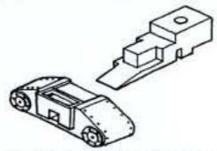
Converts 'Ibertren' to 0-4-0 or 0-4-2 with narrow gauge sized cylinders. Trailing wheels **NOT** supplied.
