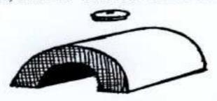
A one peice solid casting to fit a 9mm boiler, with tank filler
