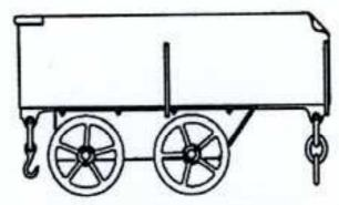
This design has an all welded body and under frame. The body has square botom corners. The kit is of all etched construction.
