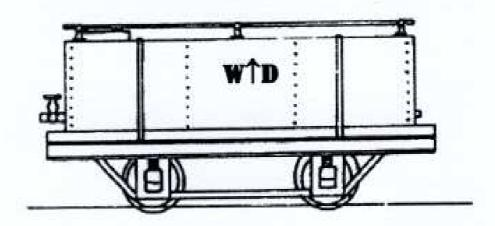
A 4-wheel tank wagon based on a World War 1 supply railways 'field' conversion, due to unstable track laid on soft ground certain locomotives with a high centre of gravity were prone to rolling over. Some had their side tanks removed and placed on flat wagons to become tenders. Our model can be used in this or similar role, or as a general-purpose tank wagon.
