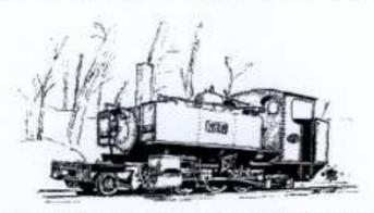
Built at the Cooke Locomotive works in 1917 for the L.R.O.D, these locos were used to supply railway lines during WW 1. A total of 100 were constructed to a British requirement and were known by their crews as 'Cookes'. They were the most powerful of the locos in service on the light railways. Similar in design to the numerous Baldwin built 4-6-0's, the Alco's wheel arrangement meant they ran equally well in either direction.
