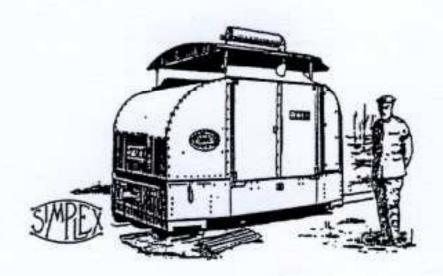
Used by the L.R.O.D during WW 1 on the forward area supply railways the loco body was built from armour plate. Similar in design to the fully armoured version (see our kit MM 1). The loco had a steel roof and deflector screens to offer protection from small arms fire and shrapnel. The most numerous of the WD 40hp 'Simplex' series, over 200 were built. Sold off as war surplus, some of these locos went into industry. At least 3 protected types are currently preserved.
