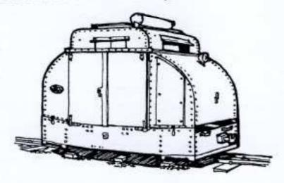
Used by the L.R.O.D during WW 1 on the forward area supply lines, the loco bodies were built from armoured plate to protect the driver against small arms fire and shrapnel. These were later sold off as war surplus and used on light railway such as Leighton Buzzard, the Festiniog Railway and at Knostrop Sewage Works, Nr Leeds. At least 5 locomotives of this type have been preserved.
