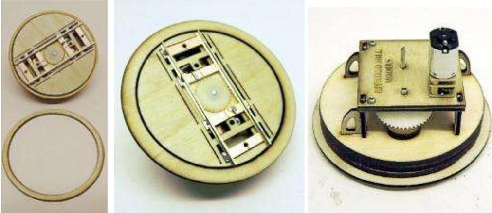
**The surface of the keeper ring is at the right height to support the incoming rail – that would be a reason to choose code 100 if you are using Peco O-16 (On30) track.**
